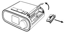
2. If applicable, place a dry, reusable blue pollen filter (1) on top of a new, optional disposable light-blue ultra-fine filter (2) and firmly snap them together.
