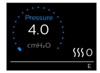
Your device has two ramp modes. Your provider will select the one that is most appropriate for you. The standard ramp mode increases pressure at a steady rate. Alternately, the SmartRamp mode maintains a constant lower pressure until the device detects that you require more pressure.
