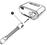
2. Press the tubing into place over the air outlet port until the tabs on the side of the tube click into place in the slots on the sides of the outlet port.
